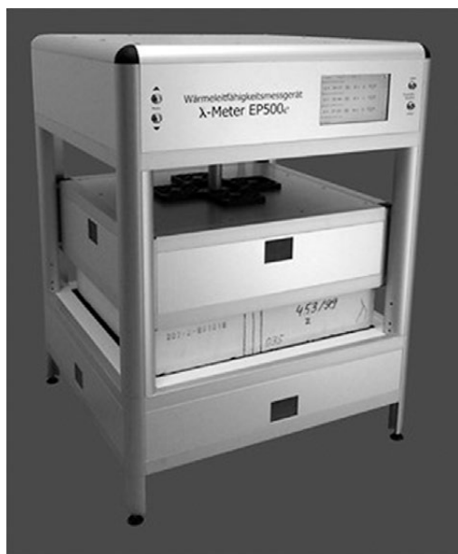
Fig. 2. Apparatus \lambda -Meter EP-500 for testing thermal conductivity
