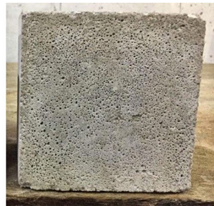
Figure 14. The surfaces of specimens subjected to elevated temperatures
