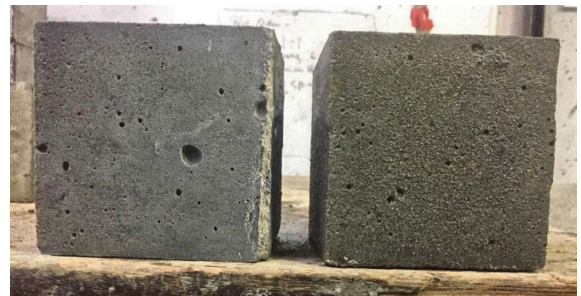
Figure 17. Appearance investigation after 28 days of immersion in HCl
