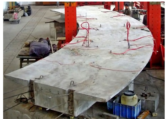
Figure 1. The large-curvature PCCBG bridge mode
